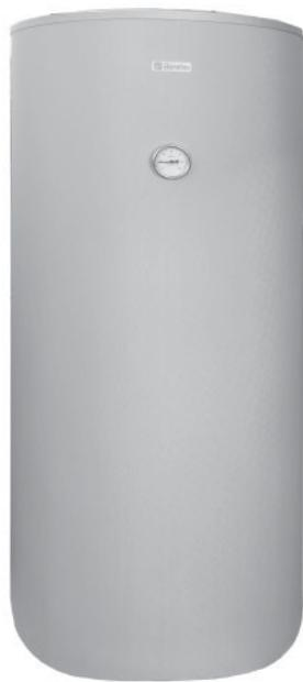
VERTICAL STORAGE DHW CYLINDERS MADE IN STEEL, PROTECTED BY A INNER ENAMEL COATING (ACCORDING TO DIN 4753), WHICH IS SMOOTH, ANTI-ADHERENT AND BACTERIOLOGICALLY INERT TO ENSURE THE ABSOLUTE HYGIENE OF THE DHW AND TO AVOID ANY POSSIBLE LIMESTONE DEPOSITS AND MAKE CLEANING EASIER. THE CARE TAKEN TO STUDY THE GEOMETRY OF THE TANK AND THE COIL (WITH A LARGE EXCHANGE SURFACE) PROVIDES THE BEST PERFORMANCE IN TERMS OF STRATIFICATION, HEAT EXCHANGE AND RECOVERY TIME.
